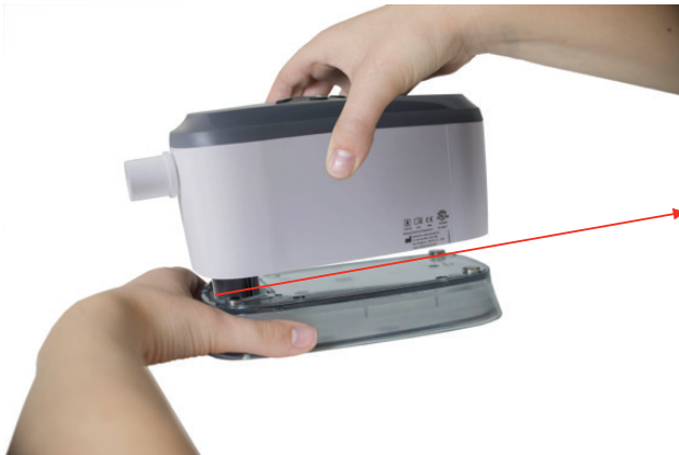
Figure 1 Line the heater cartridge up with the opening in the reservoir. Lower the device onto the reservoir. Magnets will engage to hold the two parts together.
