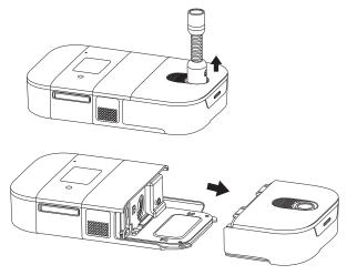
Remove the tank lid by pulling up on the tank lid tab while holding the tank base. Pour out any remaining water and rinse the tank base.
