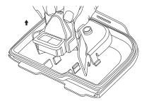
2. Remove the baffle (2) by pressing in on the side tabs and pulling up on the baffle.
