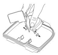
Reassemble the manifold. Align the manifold with the hooks on the tank lid. Gently press down on both manifold blocks until they snap into place.
